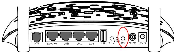
Step 2: Press and hold the WPS button of the adapter directly for 2 or 3 seconds.
