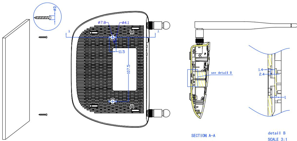
Figure 2-1 Wall-mount Install
